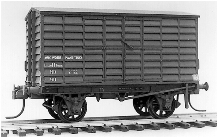
Model illustrated has been fitted with handbrake, shunter's steps and couplers (not included).
